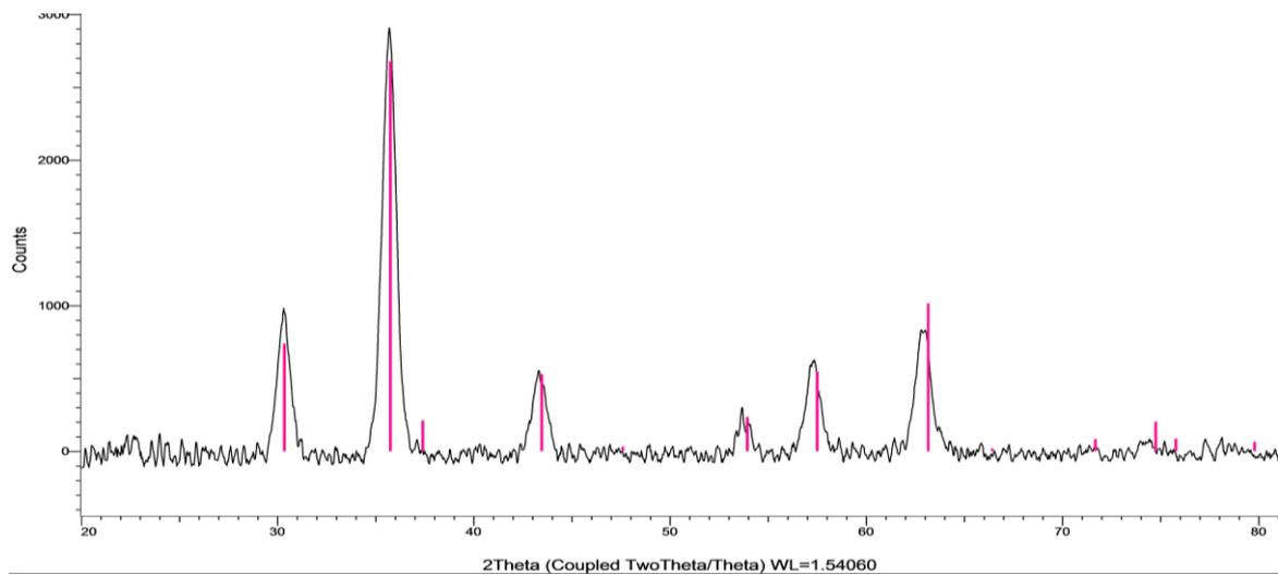
**Fig. 1. XRD of synthesis of Fe<sub>2</sub>O<sub>3</sub> nanoparticles**
